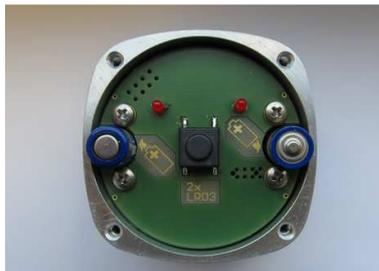
c) take off the cover and remove discharged batteries
