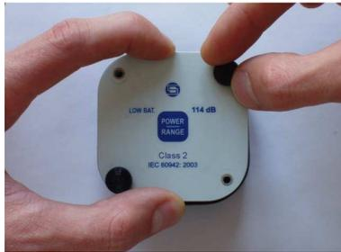
b) holding the cover unscrew four fixing screws with your fingers
