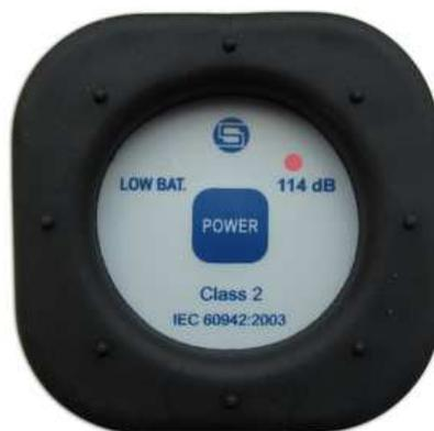
Picture 4. The top view of the SV 34 calibrator with one diode on
