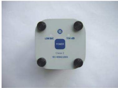
a) remove the rubber cover on the button and diodes' side
