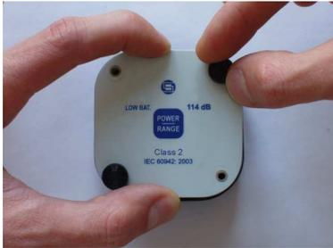
f) holding the cover with one hand fasten the fixing screws
