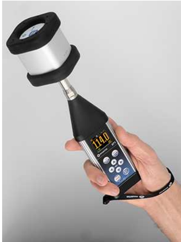
Picture 2. Calibration of the SVAN 971 sound level meter with a ½” measurement microphone
