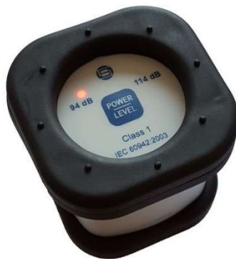
Picture 4. The top view of the SV 35A calibrator with one diode on
